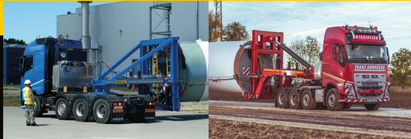
Lifting adapter with mechanical lifting equipment for 3- or 4-axle truck (depending on permitted axle load)
